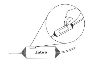
3 Connect a standard micro USB cable to the Jabra LINK 14201-33 and the PC\*.
